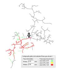
Figure 3 – Fault Location in the feeder Anita Garibaldi
